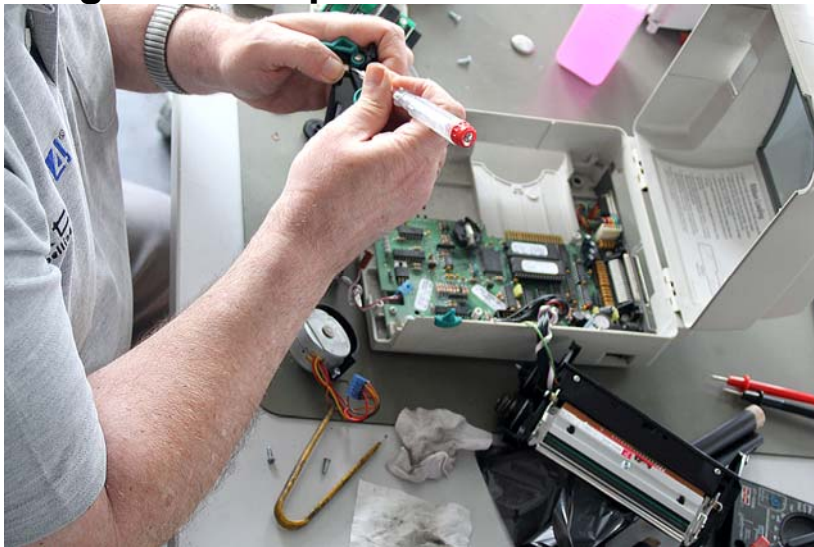
Fig.1: Repair check of a defective old thermal transfer printer
