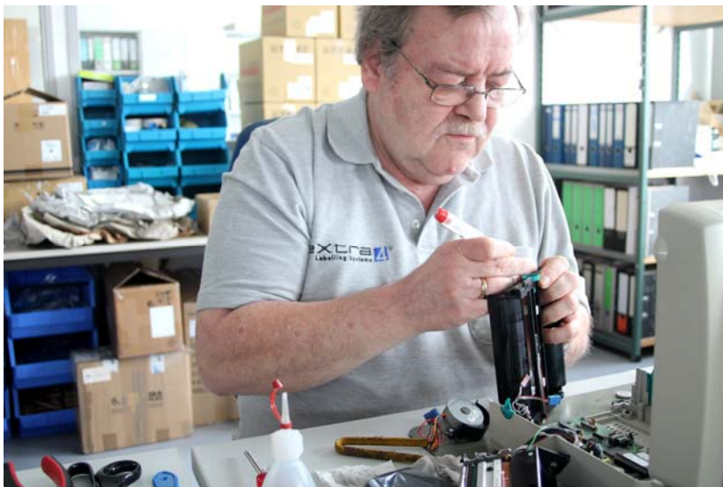
Fig.2: eXtra4 technician Hartmut Kasper disassembles a thermal transfer label printer in need of repair
